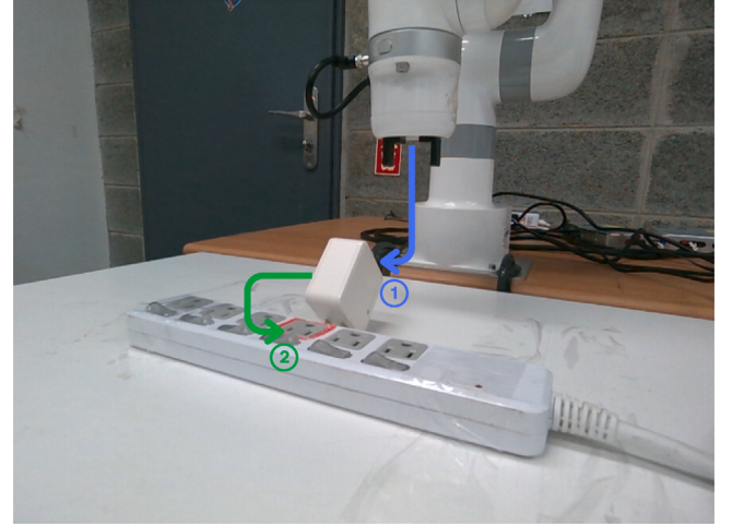
Fig. 13. Plug Insertion task. This task involves: (1) picking up a power adapter, (2) bringing it to a plug and inserting it completely.
